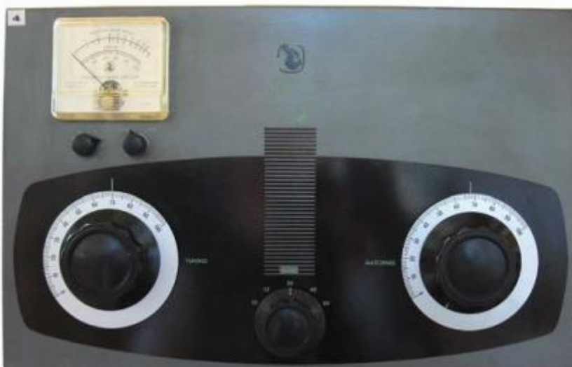
Figure 4 — A Johnson Match-box balanced-line antenna tuner from the 1950s. [Hank Garretson, W6SX, photo]
